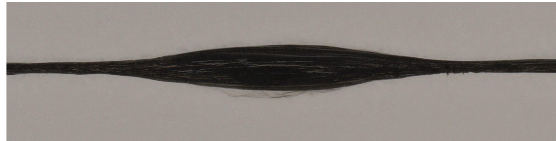
CNT yarn after beam irradiation @ HIRADMAT
